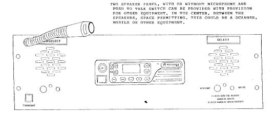
UNDER SPECIAL QUOTE, THIS PANEL IS AVAILABLE WITH TWO SPEAKERS, WITH OR WITHOUT THE MICROPHONE AND PUSH TO TALK SWITCH.
